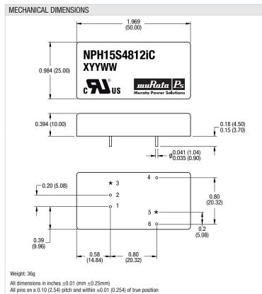
The copper case is internally connected to the output (-Vout) pin. Care is needed in the design of this circuit board on which the converter is mounted. Top side tracks must not contact the edge of the case or the ferrite core, visible on the underside of the unit.
